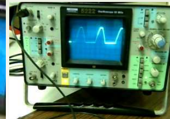
2) effet diode (redressement mono-alternance)
